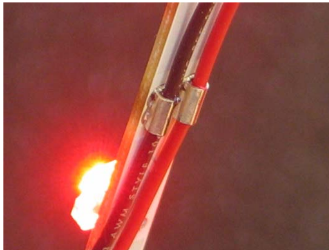
Figure 10: A vertically oriented PCB, two "pass-through" wires, two crimp terminals and a glowing LED
