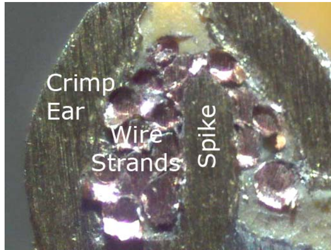
Figure 8: A cross-section view of a wire inserted into the Crimp Terminal. Note that the spike solidly penetrates the wire strands.
