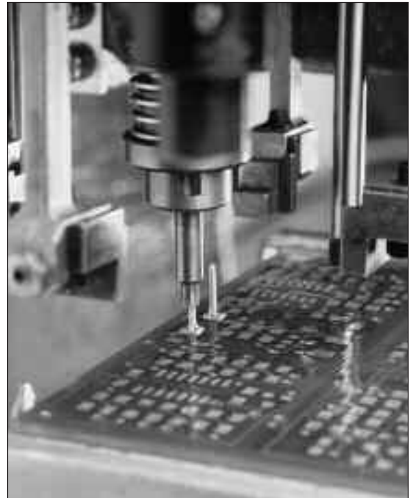
Odd-shaped parts can now be assembled in-line on existing placement equipment.
