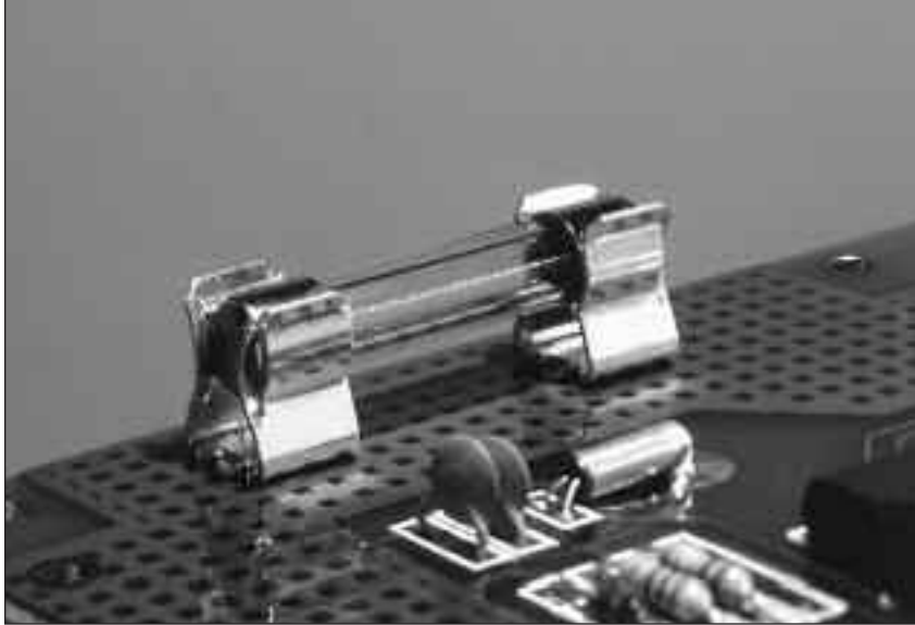
Zierick's spring-loaded mounting technology provides improved retention in Snap-In fuse clips.
