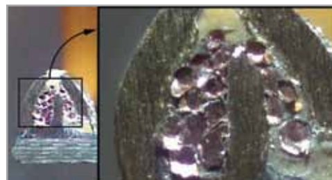
Figure 5: Cross Section of Terminated Wire
