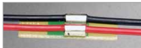
Figure 3: Wires Properly Terminated by the Press
