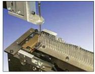
Feeder capacity is 24" of the header strips. New strips can be loaded on
